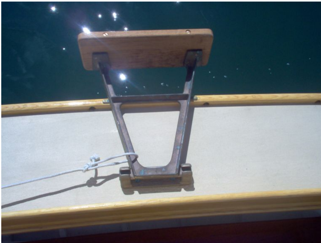
Outboard Bracket With Bronze Strip Protecting Toerail
